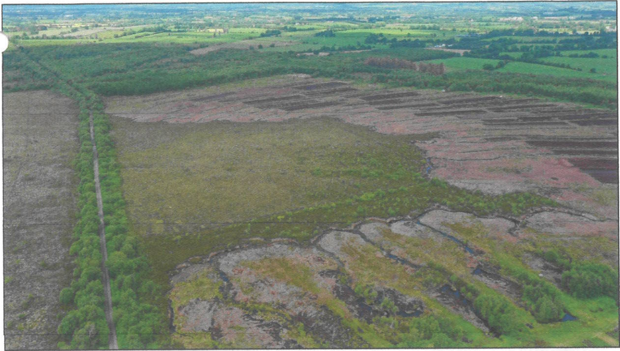
Figure 1: DRAINAGE AND PEAT REMOVAL FROM NORTHERN SECTION OF BOG
